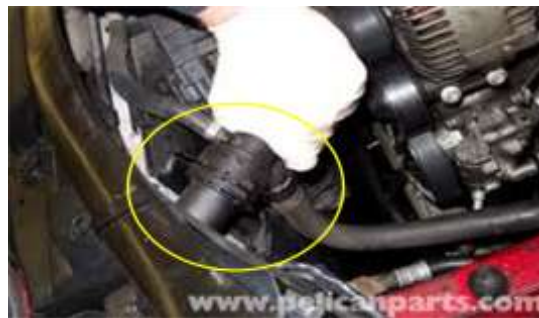
Fig. 2 Quick connector used in Automotive cooling
